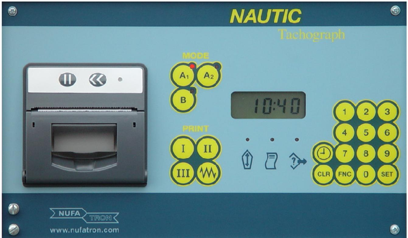
Normally the display of the **NAUTIC-Tachograph** shows the actual time and the selected operation mode.
